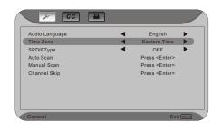
SPDIF Type-Setting the coaxial type to PCM off or Dolby digital.
